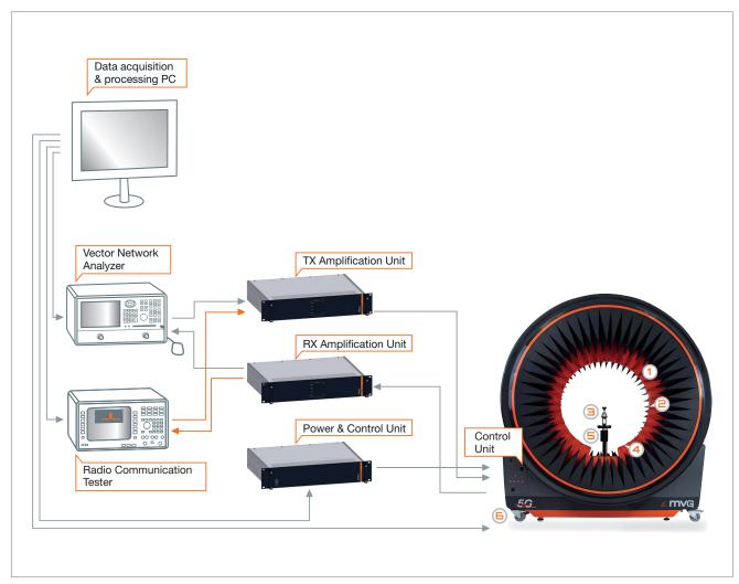
The StarLab 50 GHz is an all-in-one, turnkey test system solution which comprises the probe array unit as well as the necessary controllers, RF units, and software. The SL control unit drives the two positioning motors of the device and the electronic scanning of the probe array. The subsystem power and control unit supplies the power and drives the RF units. The amplification units convert
