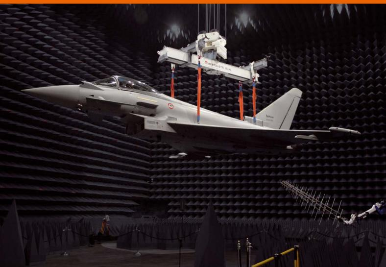
String Reel Target Manipulation Systems are used to support targets for low frequency Radar Cross Section (RCS) measurements. Three sizes of string reel positioners are used to handle various loads from scaled models to full size targets. Another use is for manipulation of a calibration target in anechoic chambers. A typical application requires 3 - 16 string reel positioners for the various loads.
