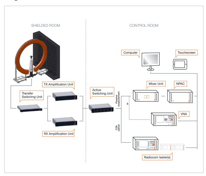
SG 64 uses analog RF signal generators to emit EM waves from the probe array to the antenna under test (AUT) or vice versa. It uses the NPAC as an RF receiver for antenna measurements. The NPAC also drives the electronic scanning of the probe array. The NPAC includes the fastest and most accurate sources and receivers on the market.
