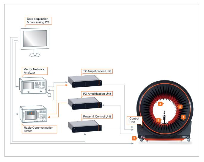
The StarLab 50 GHz is an all-in-one, turnkey test system solution which comprises the probe array unit as well as the necessary controllers, RF units, and software. The SL control unit drives the two positioning motors of the device and the electronic scanning of the probe array. The subsystem power and control unit supplies the power and drives the RF units. The amplification units convert low power to high power radio frequency signals via the transmission and reception channels.
