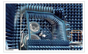
Most horns are available in single and dual linear polarization. Circular polarization is typically calculated from two linear polarizations, but also circular polarized feeds can be used.
