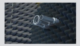
In the most common compact range reflector systems, a large reflector is illuminated by a feed to ensure that the amplitude and phase variation is minimal across the Quite Zone (QZ). To avoid obstruction by the feed an offset reflector geometry is used. This offset geometry causes a cross-polarization as a function of position in the QZ.
