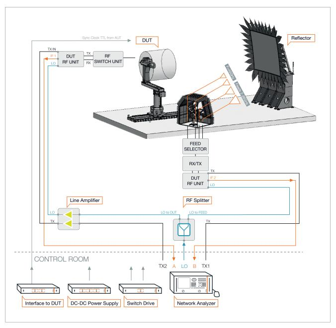
The lowest operational frequency of a compact range system is detemined by the size of the reflector, the edge treatment and the absorbers.
