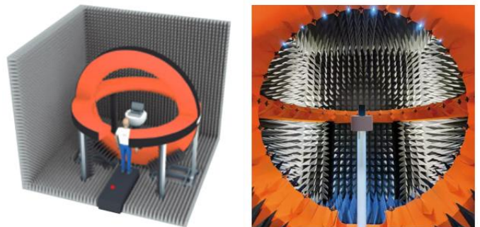
Figure 1. Measurements of MIMO OTA performances using a typical MPAC solution based on a horizontal ring of probes.
