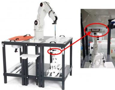
Fig. 2. GWD radiating in proximity of a phantom system in the MVG ComoSAR system [4].
