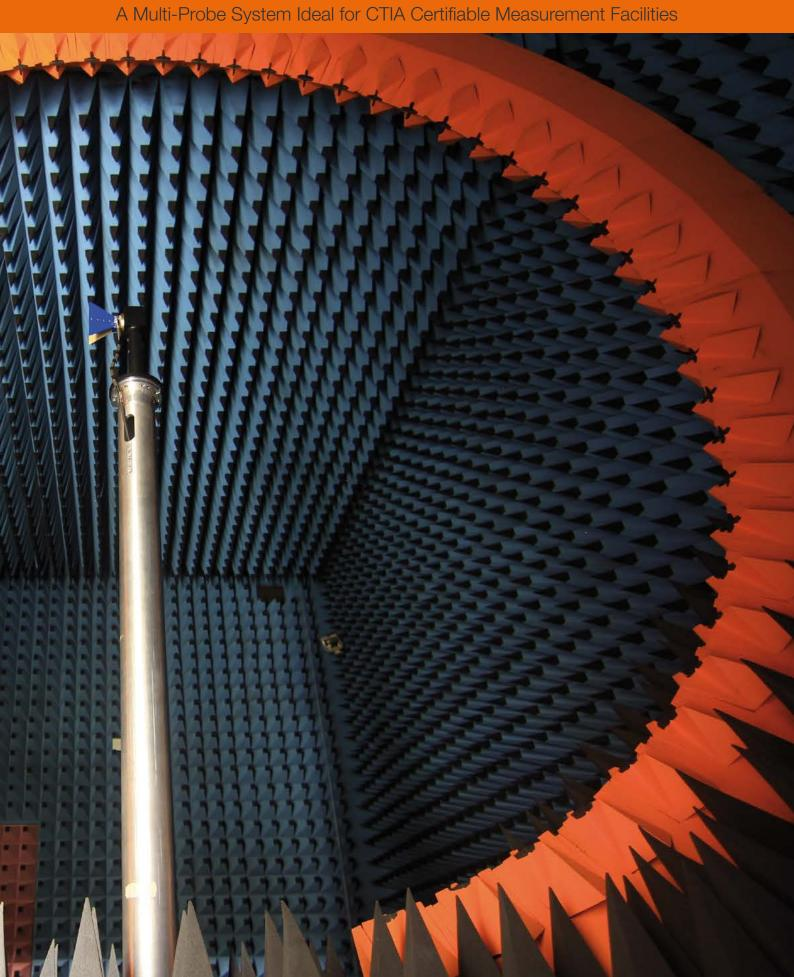
The most accurate solution for testing antennas and wireless devices: SG 64 has been developed to measure stand alone antennas or antennas integrated in subsystems. It is also ideal for CTIA certifiable measurement facilities.
